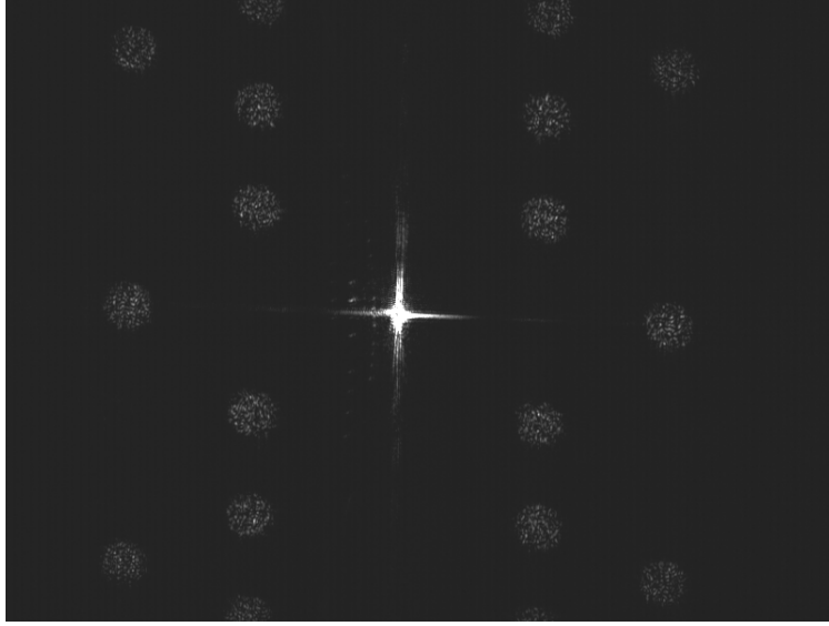
Figure 4.25: Phase Hologram vs Phase Grating: The far field image created with a phase hologram loses intensity in each beam but all 18 original beams are present and remain focussed. (The brightness and contrast levels of this picture have been enhanced by 15% for printing of this document).
